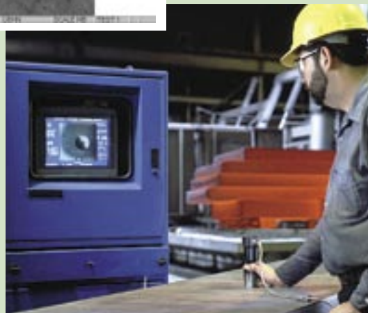
The Brinell Impression is displayed on the Lab B.O.S.S. monitor so the operator can position the test head properly for measurement.
