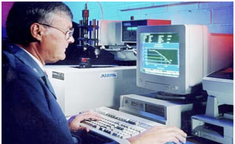
Carolina Commercial Heat Treating metallurgist and quality control manager Jack Grochowski checks the microhardness vs. case depth graph generated by an MT90 after testing a heat treated part. The Newage Testing Instruments' system automatically calculates effective case depth for up to three Rockwell-scale test values and verifies that they fall within predefined limits
