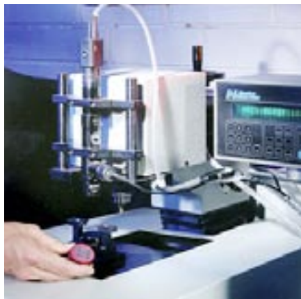
A specimen mount containing polished cross sections from nine heat treated parts can be microhardness tested at one time using the MT90. The operator must first visually locate the edge and orientation of each section on the instrument's monitor. The MT90 computer can then run all nine traverses sequentially without further operator interaction. Note that different, predefined traverse setups can be used for the sections contained in a single mount.
